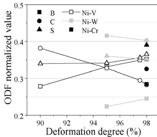
Figure 1 ODF values for B, C and S components (square, circle and triangle, respectively), relative to the total  $\beta$ -fibres values, vs. degree of deformation for Ni-V (open symbols), Ni-W-Cr (black) and Ni-W (gray)
