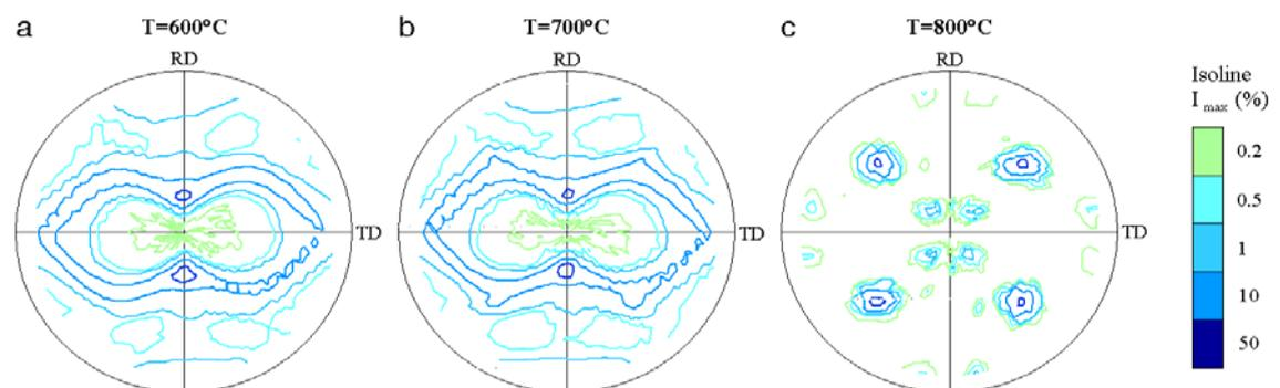
Figure 2. (111) pole figures for three Ni-W samples annealed at (a) 600, (b) 700 and (c) 800 °C and then quenched to room temperature. Non-cube reflections at 800 °C refer to  $\{221\} \langle 122 \rangle$  orientations were observed.
