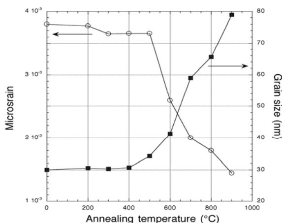
Figure 4. Evolution of microstrain (empty dots) and grain size (full squares) for Ni-W samples annealed at different temperatures and quenched to room temperature, evaluated by Monte Carlo procedure on  $\theta$ -2 $\theta$  diffraction peaks.
