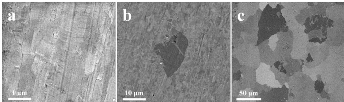
*Figure 5. SE (a) and BS (b-c) SEM images of Ni-W sample annealed at (a) 600, (b) 700, and (c) 800 °C and quenched to room temperature.*
