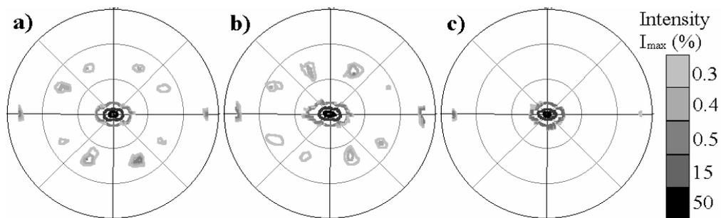
Figure 8. (002) polar figures of  $\text{Ni}_{89}\text{V}_{11}$  (a),  $\text{Ni-5at\%W-5at\%Cr}$  (b) and  $\text{Ni}_{95}\text{W}_3$  (c) tapes recrystallized at 900°C for 4 hours in vacuum ( $10^{-7}$  Torr); isolines are set in order to underline the presence of twins.
