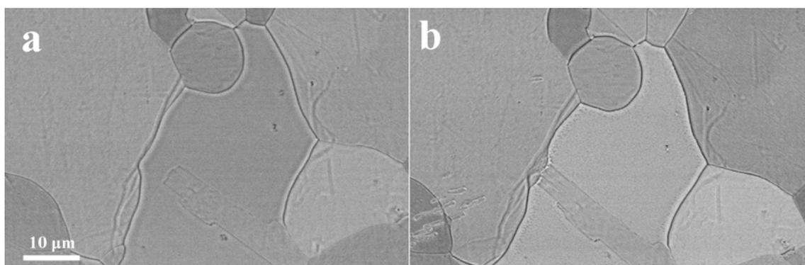
*Figure 7. BS-SEM images at the same magnification of a Ni-W sample recrystallized at 900 °C for 5 minutes, before (a) and after (b) simulation treatment at 850 °C for 30 minutes.*
