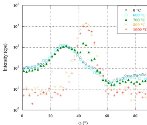
Figure 3.  $\varphi$ -scans at  $\chi=54.7^\circ$  for (111) pole figures of Ni-W samples annealed at different temperatures shown in figure 1. The appearance of a peak at  $\varphi=45^\circ$  for the sample annealed at 700 °C indicates the beginning of recrystallization. Intensities are plotted in logarithmic scale in order to enhance low intensity reflections.
