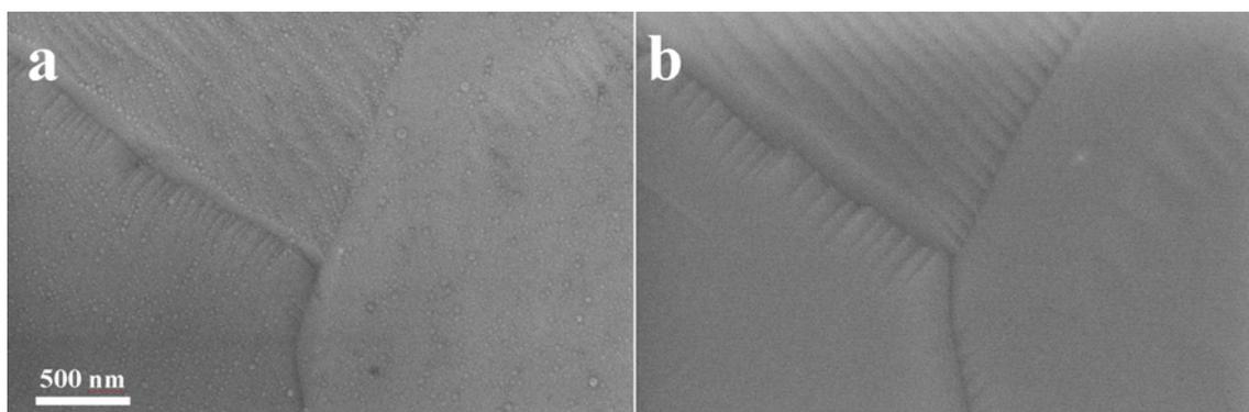
*Figure 6. SE-SEM images at the same magnification of a Ni-W sample recrystallized at 900 °C with no plateau, before (a) and after (b) simulation treatment at 850 °C for 30 minutes. Low-angle grain boundary migration can be estimated.*
