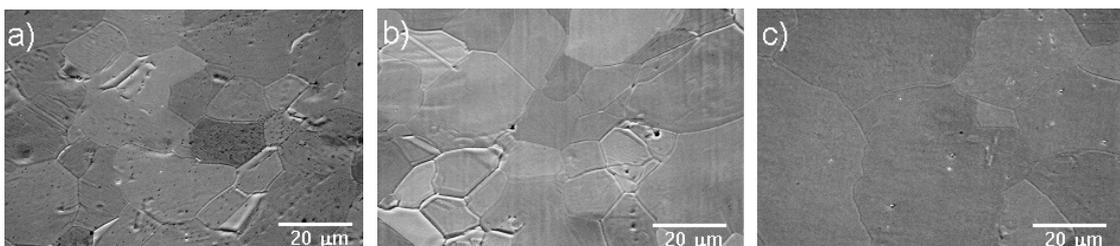
Figure 9. SEM micrographs of Ni-V (a), Ni-W-Cr (b) and Ni-W (c) tape surfaces
