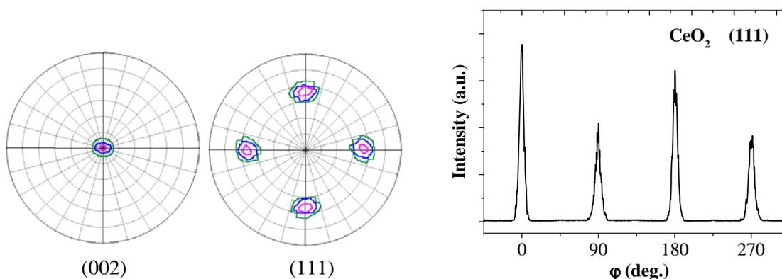
Figure 11. (002) and (111) pole figure of 500 nm CeO<sub>2</sub> film on Ni<sub>95</sub>W<sub>5</sub> substrate and  $\phi$ -scan (111); in pole figures equiangles are in logarithmic scale.
