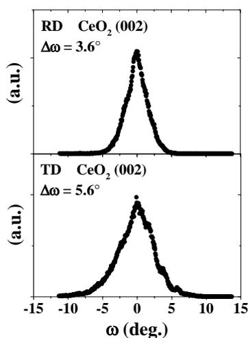
Figure 10. Rocking curves for the (200) peak of CeO<sub>2</sub> on Ni-W substrate
